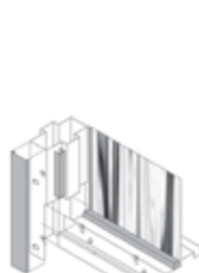
SILL / MULLION DETAIL WITH GLASS STOP
